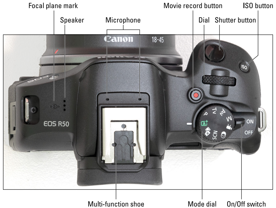
FIGURE 1-10: Here's a guide to controls found on top of the camera.
