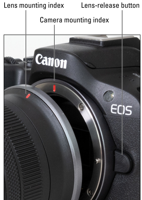
FIGURE 1-3: Align the red mounting index on the lens with the one on the camera body.
