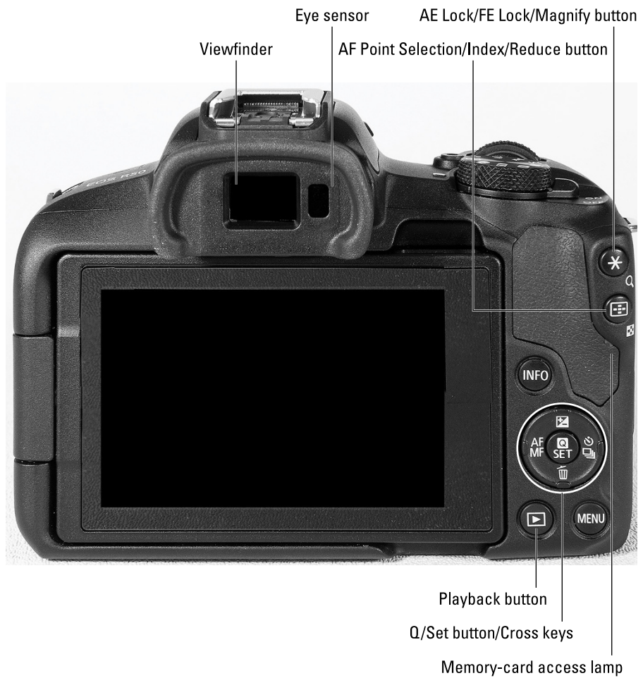
FIGURE 1-12: Having lots of external buttons makes accessing the camera's functions easier.
