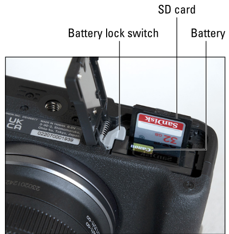
FIGURE 1-2: The battery and memory card go into the compartment on the bottom of the camera.
