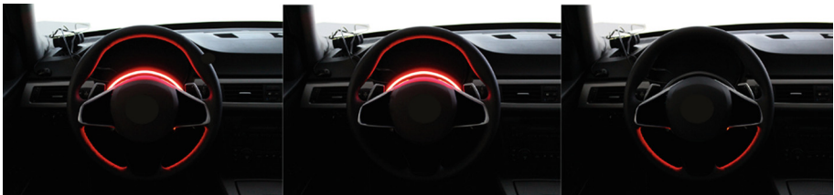
Fig. 4. Experiment conditions with full rim, upper rim only or lower rim only illumination on the steering wheel, integrated in the driving simulator cockpit. In the baseline condition, there was no (visual) warning at all.
