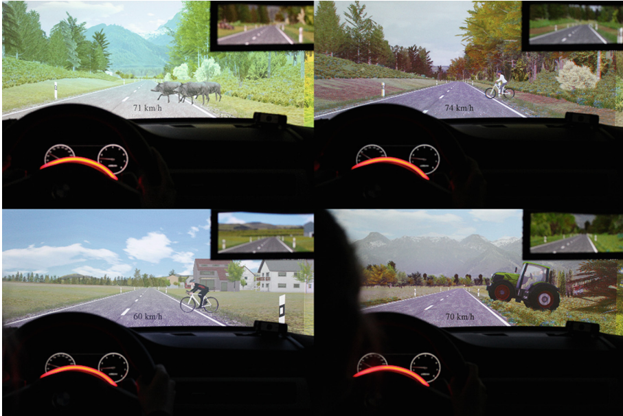
Fig. 6. Visual warning with BRLE highlighted and four different collision objects: wildboars, cyclist, mountain biker and tractor
