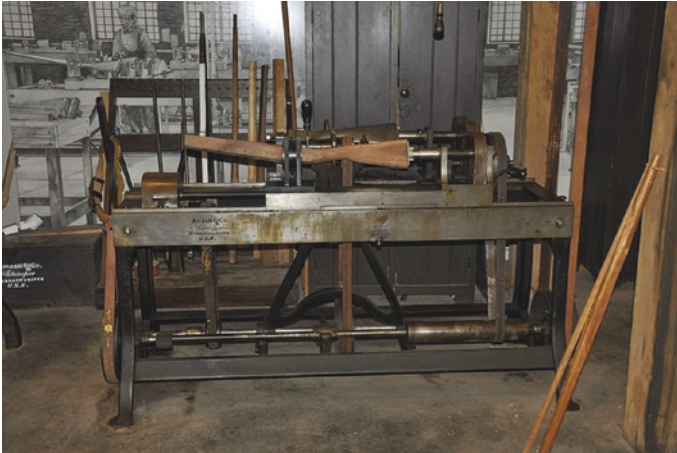
Figure 2. A Blanchard lathe, with gun stock on the machine ( https://commons.wikimedia.org/wiki/File:Harpers_Ferry_gun_smith_shop_-_Blanchard_lathe_-_01.jpg )
