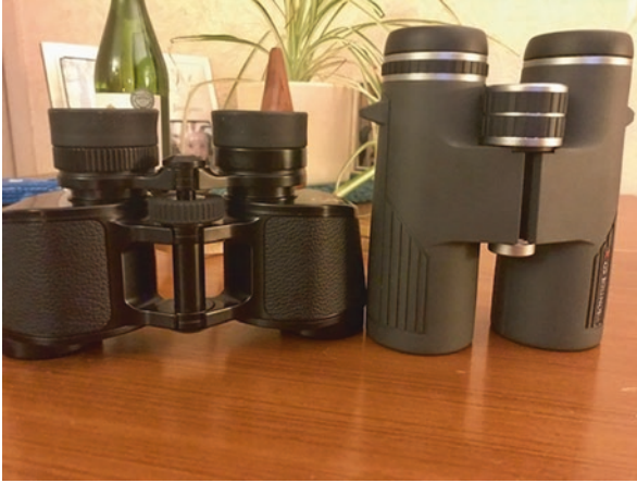
Two binocular designs: a Porro prism instrument (left) and roof prism model (right)
