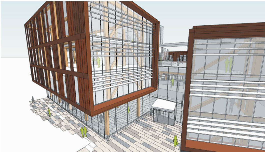
Figure 1.3: Architectural design visualization model that was used to evaluate various shading solutions for an academic building. (Image used with permission of Leers Weinzapfel Associates)
