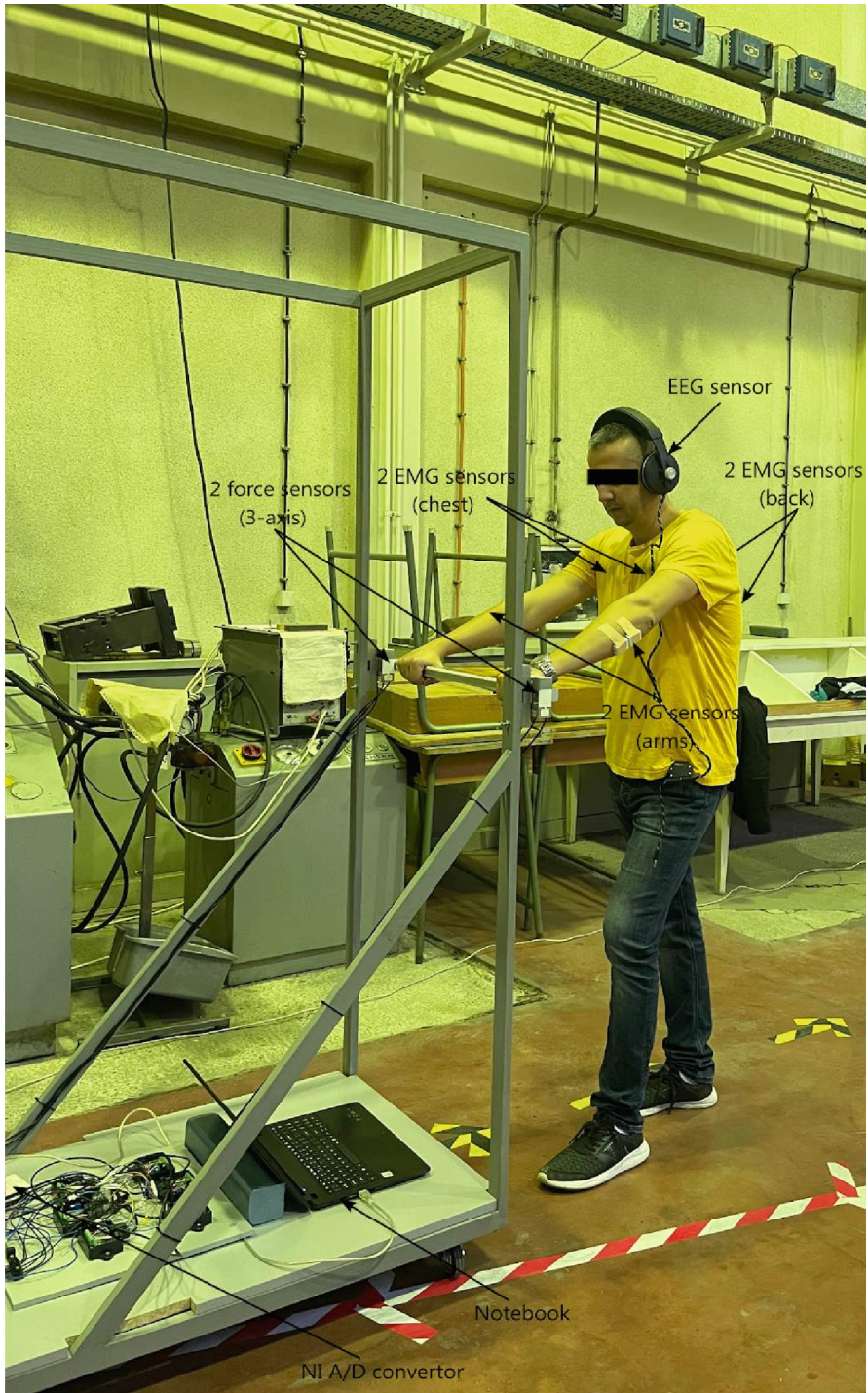
Fig. 8. Experimental setup for P&P task
