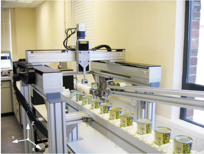
Figure 1.1 A gantry robot for a pick-and-place operation with the axes marked.
