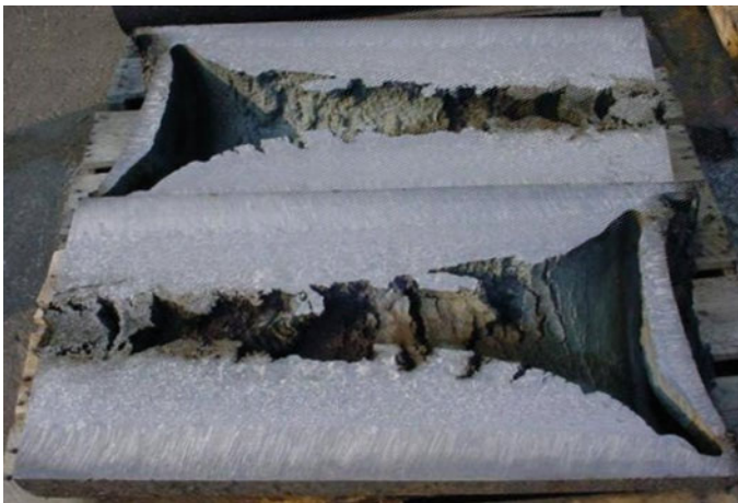
Fig. 2 Shrink pipe from a statically cast VIM electrode
