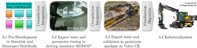
Fig. 2. Toolchain in the development process of the stability assistant for wheeled excavators: From an offline predevelopment phase (Section 3.1) and online expert tests in the driving simulator RODOS® (Section 3.2) at the Fraunhofer ITWM to further expert tests in a prototype machine (Section 3.3) and the industrialization (Section 3.4) at Volvo CE.
