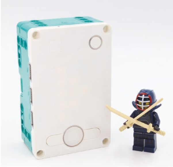
Figure 1-1. The Hub is a small computer for controlling sensors and motors
