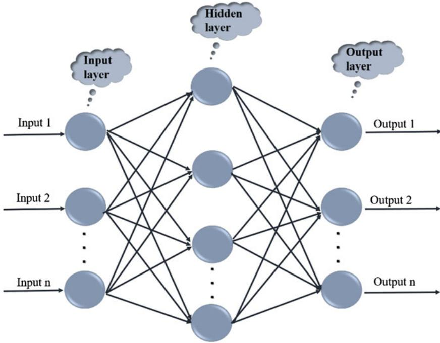
Fig. 5 Structure of an artificial neural network
