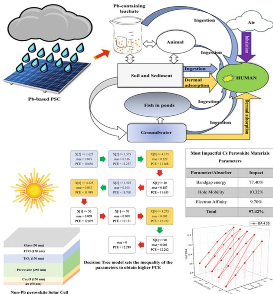
Fig. 7 Machine learning approach to delineate the impact of material properties on physics of solar cell device. Reprinted with permission from Ref. [37]. Copyrights 2022 American Chemical Society
