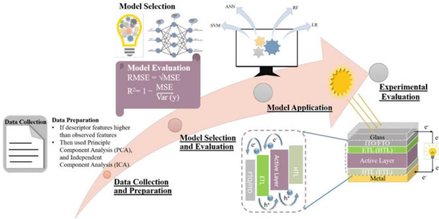
**Fig. 3** The general workflow of ML for solar cells includes data collection and feature engineering, model selection and evaluation, model application, and experimental evaluation
