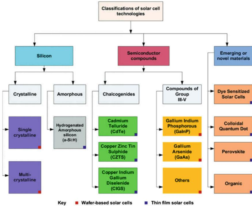
**Fig. 1** Classification of solar cells. Reprinted with permission from Ref. [5]. Copyrights 2017 Elsevier
