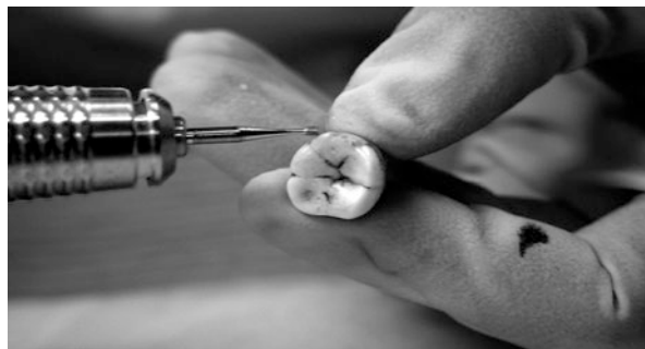
Fig. 1.3 Sampling tooth enamel. The first step is to lightly grind the surface of the enamel to remove potential contamination
