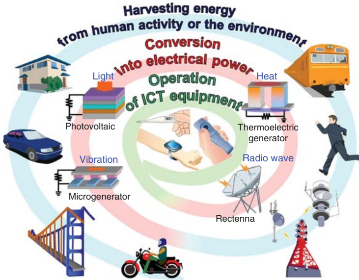
Figure 1.1 Schematic illustration of energy-harvesting strategies based on the ambient energies [2]. Source: Reprinted with permission from Fujitsu Laboratories Ltd. [2]; © 2016 MEMS consulting.
