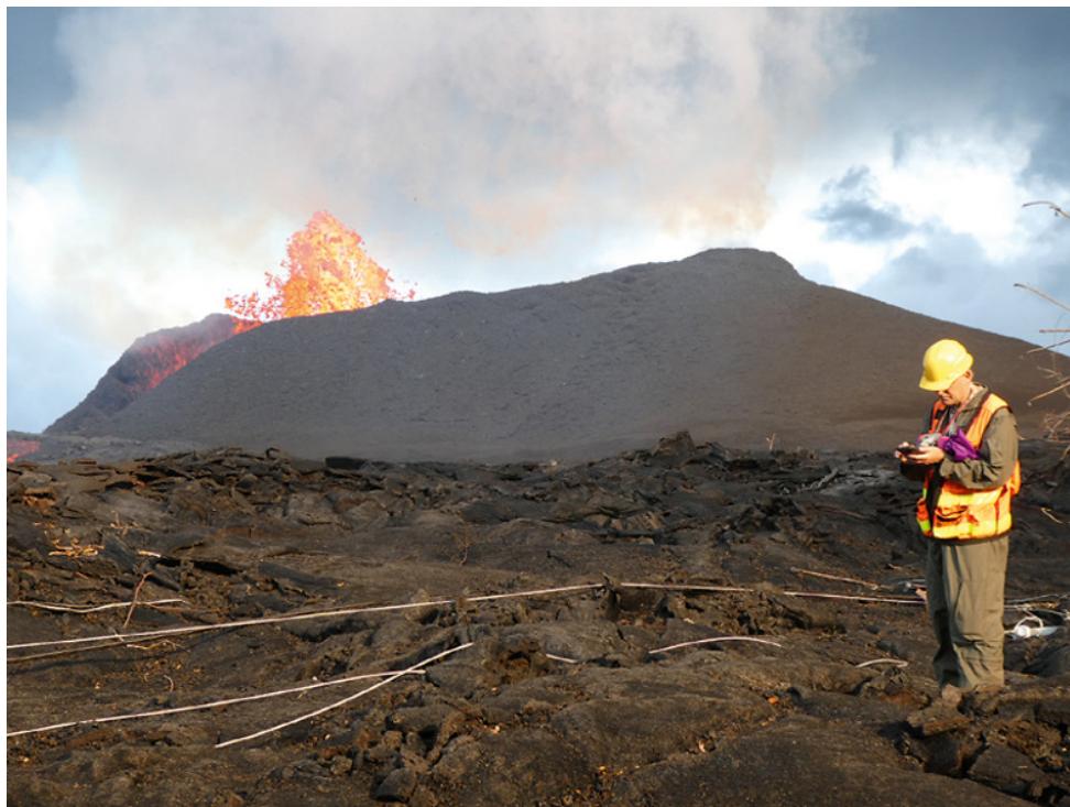
FIGURE 1.7 Trigonometry works! Measuring the height of a lava fountain within with a GPS and inclinometer. Fountains rise about 60 m above the base of a freshly forming cone (Fissure 8) in Leilani Estates. This cone has since been named Ahu’ailā’au by Hawaiian elders, meaning “Altar of Ailā’au” (a vindictive Hawaiian volcano god before Pele). Downed power lines and electric cables litter the landscape. Source: USGS photo by Samantha Gassett.
