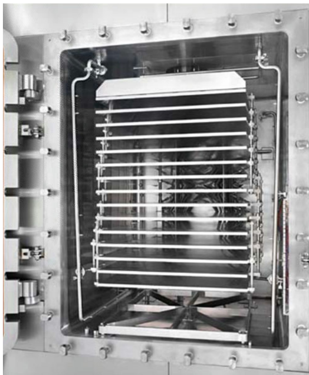
Fig. 1 Freeze Dryer Chamber with shelves. (Courtesy SP Scientific)
