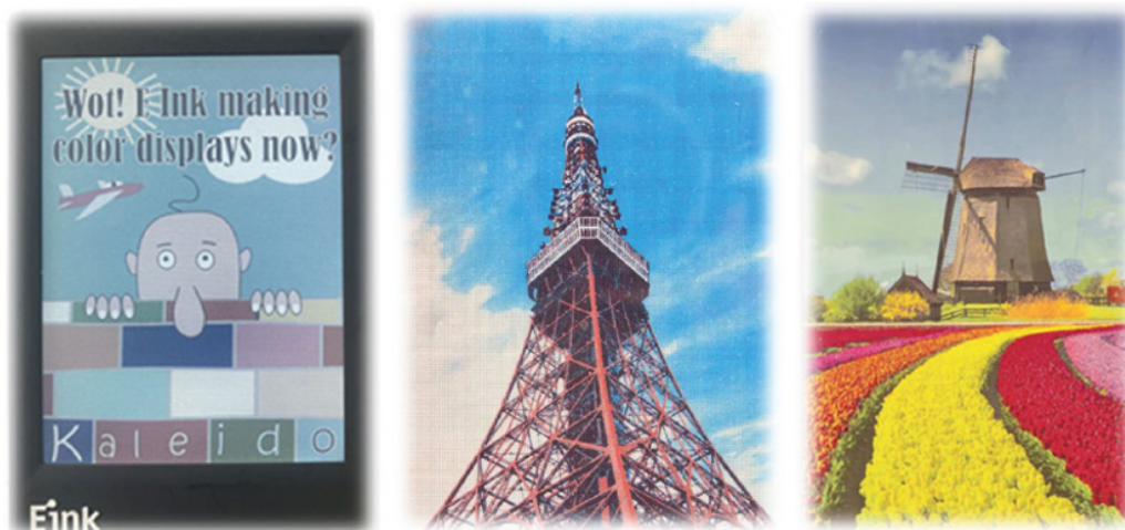
Figure 1.9 Prototypes of colored electrophoretic displays: the left image uses a color filter and front light, while the middle and right images use the multiple color particles design [16–18] A. [18] Ian French, et al. 2020; B.[16] Hiji N, et.al, 2012 / John Wiley & Sons, Inc.; C.[17] Telfer S J, MD McCreary, 2016 / John Wiley & Sons, Inc.
