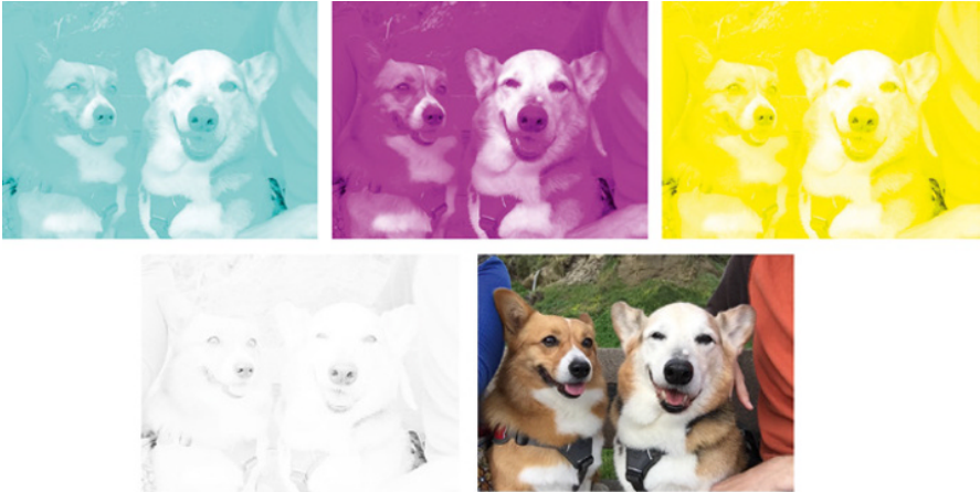
Figure 1.3 Color separation of an image into its CMYK components, and the final printed image. The absence of a color is white.
