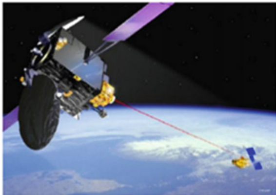
Fig. 1.10 Schematic of inter-satellite communication between GEO and LEO in SILEX [91]
