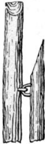
Fig. 4.—Method of Attaching Support to Easel.
