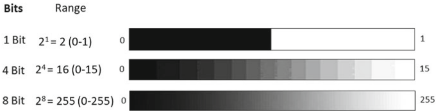
Fig. 5 The relationship between bit and the grayscale values (American Cinematographer 2005)
