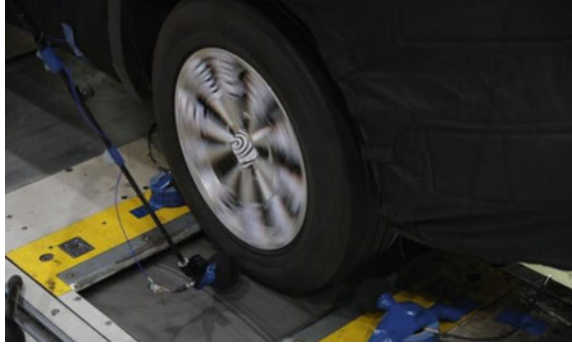
Fig. 2.8 Noise measurement of a rolling tire
