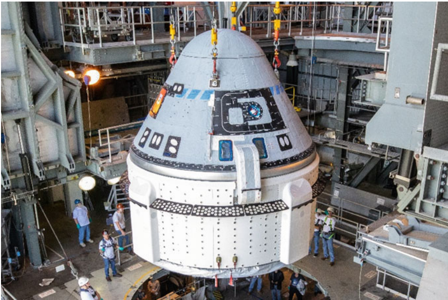
Fig. 1 A Boeing-manufactured Starliner capsule being mated with an Atlas 5 rocket. Software bugs and a telemetry issue forced the curtailment of the December, 2019, OFT1 shakedown test. Technology is fallible (Wikimedia [36])
