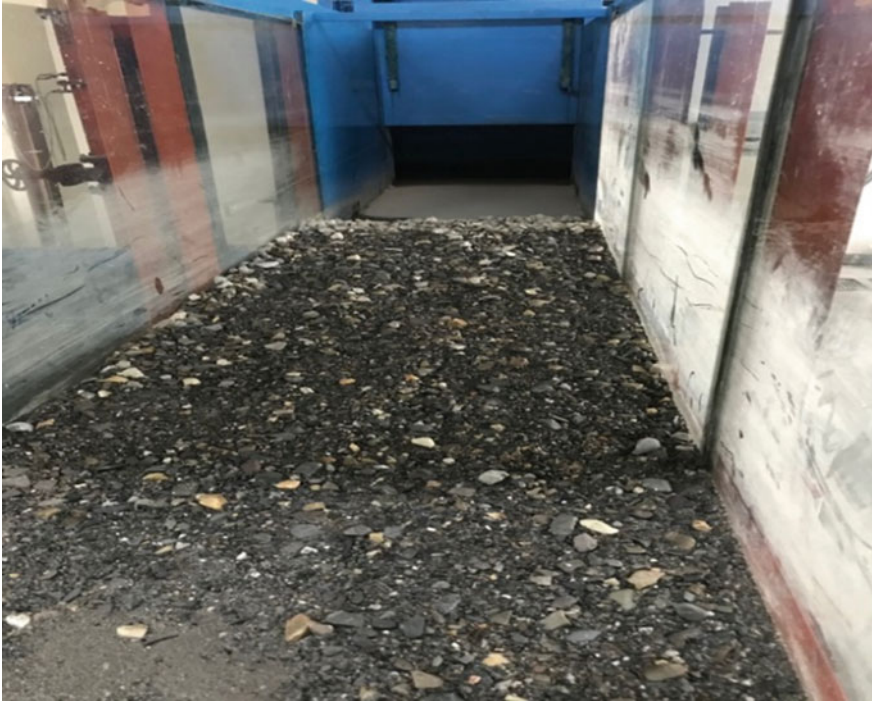
Fig. 6 Coarse aggregate laid at the water entry point in the flume to prevent erosion
