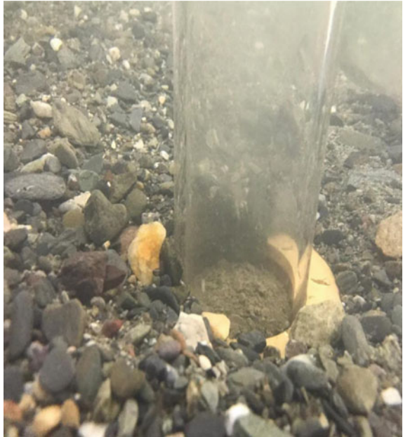
Fig. 8 Vortex formed at 4 rotations. The water strikes the pier directly and spreads up in three different directions (three-dimensional flow, time interval 10 min)
