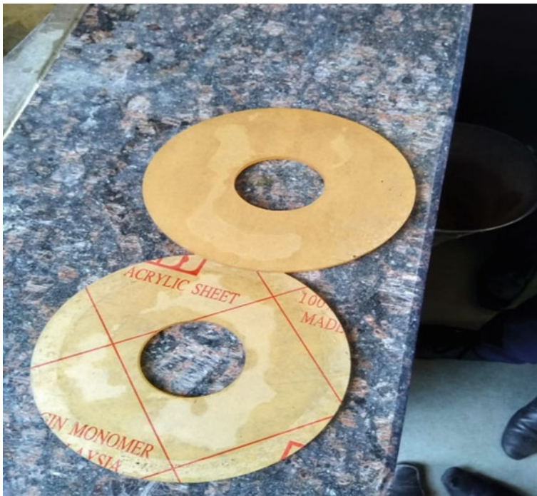
Fig. 3 Circular acrylic sheets with inner radius 50 mm and thickness of 5 mm
