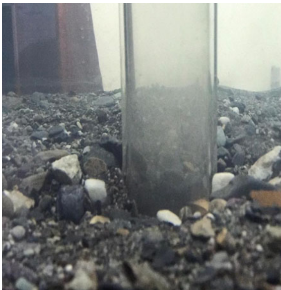
Fig. 10 Due to silting and decrease in the velocity, scour depth gets decreased (10–20 min interval)
