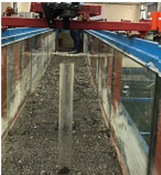
Fig. 5 Camera mounted above the pier for recording the flow pattern
