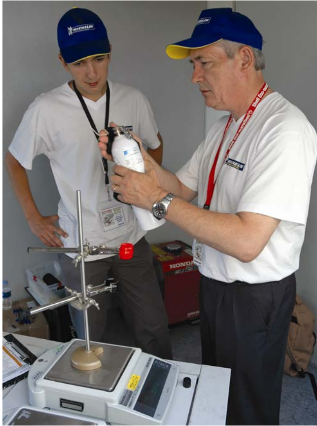
Figure 1-5: Measurement by weight of the hydrogen consumption of PAC-Car II during the Shell Eco-marathon at the Michelin Technology Center in 2005.
