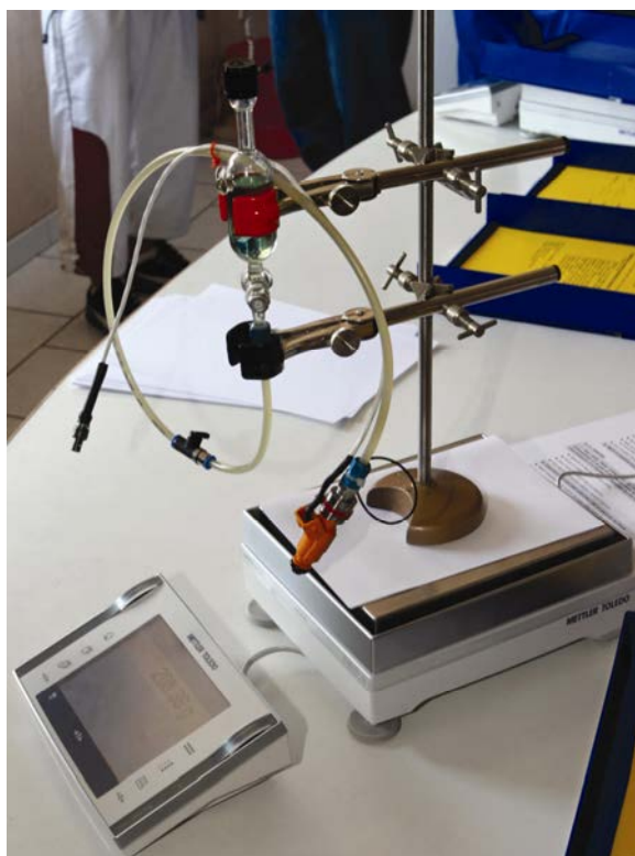
Figure 1-4: Measurement by weight of the fuel consumption during the European Shell Eco-marathon. The entire fueling system has been put on the scale. (Courtesy of Shell)
