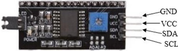
Fig. 8 Pin configuration of I2CAdapter
