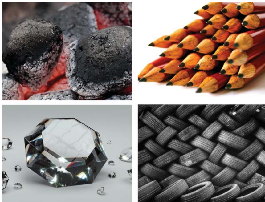
Figure 1.1 Typical carbon materials, such as charcoals, pencil lead, diamond, and carbon black–reinforced tires. Source: Pixabay.com. Reproduced with permission of Pixabay.
