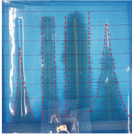
Fig. 5. Shapes of the flow front propagation as a function of the flow velocity in the impregnation channels 3 through 6
