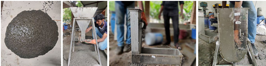
Fig. 7 Tests on fresh concrete: slump flow, V-Funnel, L-Box and U-Box test, respectively
