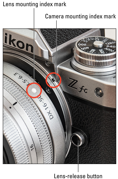
FIGURE 1-3: Position the lens so that its mounting index aligns with the one on the camera.
