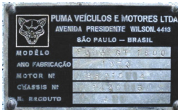
On the type plate between 1970 and mid-1972, the Puma is shown with moustache hair. The engine number and chassis number were taken from Volkswagen, the product number identifies the body
