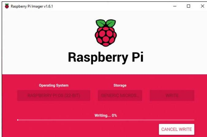
Figure 1.7: Writing to the SD card using the Raspberry Pi Imager.
