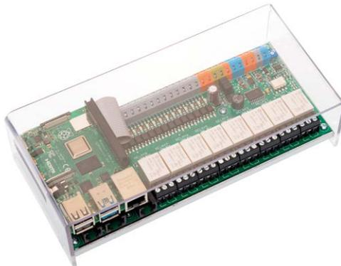
*Figure 0.1: Raspberry Pi PLC Unipi 1.1.*
