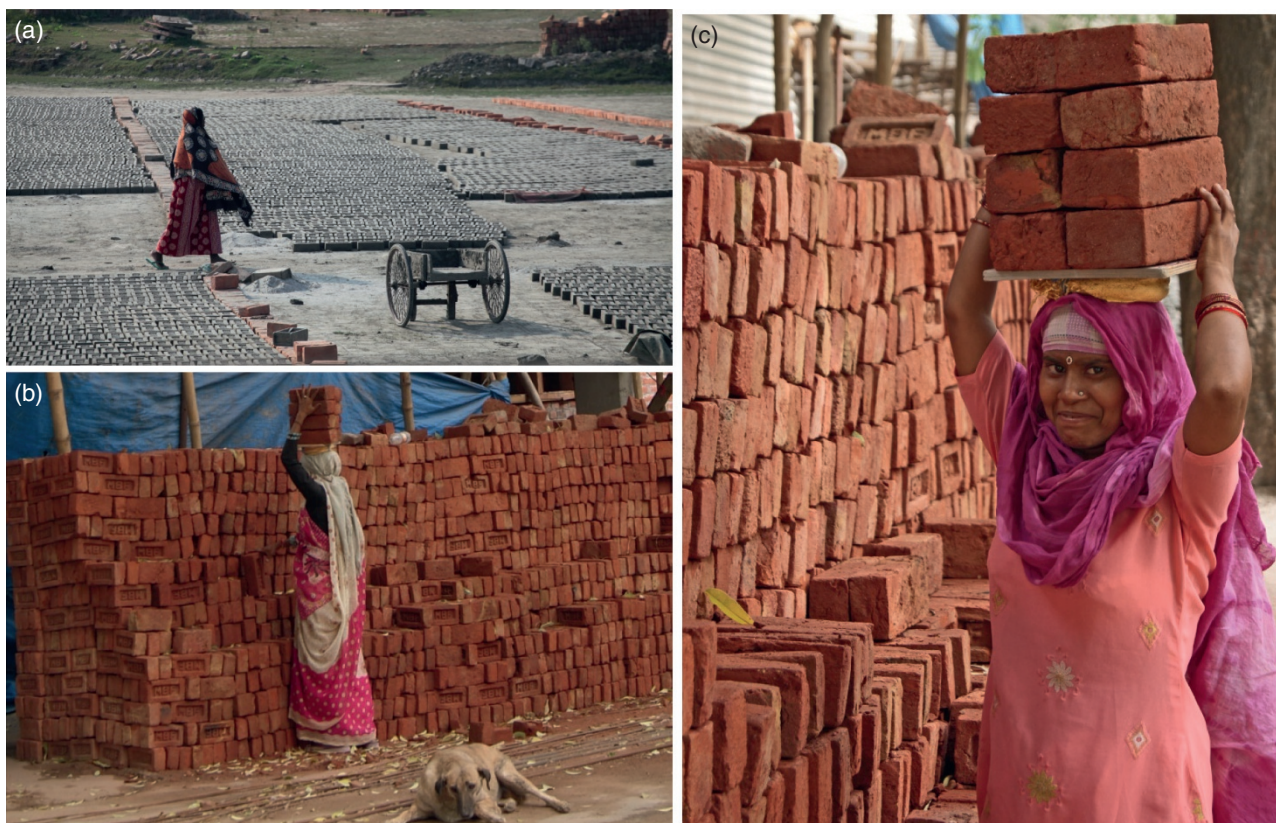
Figure 1.1 Harappan style of brick production from clay. (a) Process of sun drying of clay bricks (in Kolkata) Source: Courtesy of Sreewoshi Sinha; (b) and (c) Fired products at a construction site in New Delhi in 2010. Source: Nirmal Sinha.
