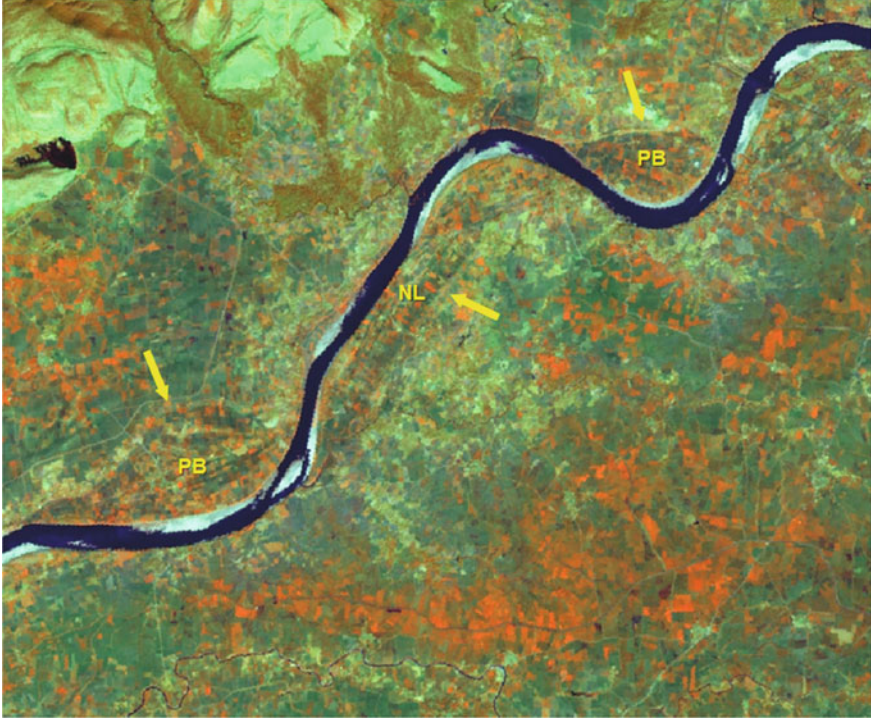
Fig. 1.2 Use of SWIR band in deriving a color composite highlights the fluvial landforms along the Tawa river in Madhya Pradesh. The color composite is derived using SWIR, IR, and Red bands were given to RGB. The landform labels are: PB-point bar, NL-Natural levee
