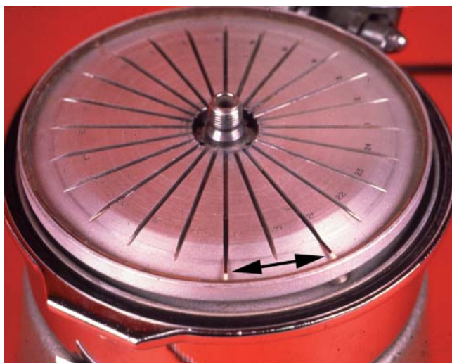
Figure 1.6 Placement of microhematocrit tubes on a microhematocrit centrifuge head. Note the proper orientation of two microhematocrit tubes, with the clay-sealed end positioned at the outer ring of the centrifuge head (double arrow).
