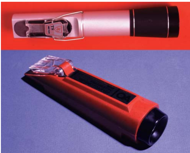
Figure 1.9 Refractometers. The lower refractometer is more rugged, because it is encased in rubber. It is known as a veterinary refractometer, and it has a canine and feline urine specific gravity scale that calibrates for minor differences between species during this determination.
