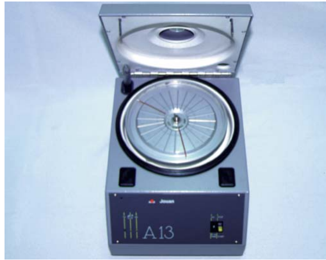
Figure 1.5 Representative microhematocrit centrifuge. The head and motor are designed to spin the tubes at very high speeds to achieve maximal erythrocyte packing.
