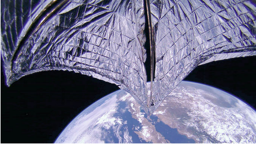
Fig. 1.1 In-space picture of the deployed solar sail of LightSail-2 mission. Credits The Planetary Society
