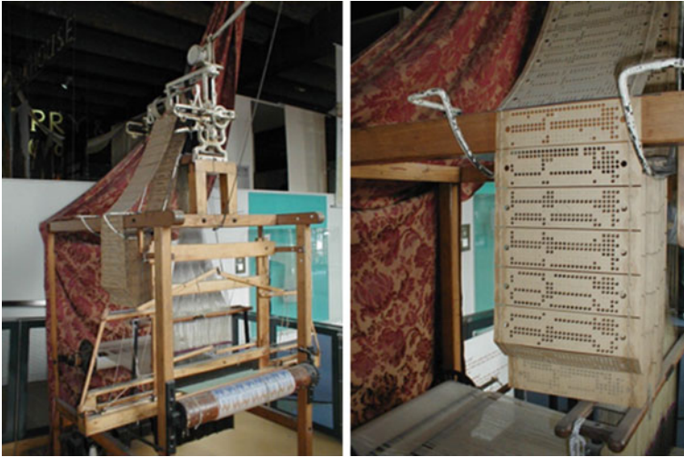
Fig. 1.1 The Jacquard weaving loom (1805) is probably the first man-made tool generating patterns from a digital Memory medium, astonishingly similar to the punch cards of the 20th cty. It continues to serve as a metaphor to explain reproducible pattern formation controlled by digital data, for example the genetic control of embryonic development [Nus04].
