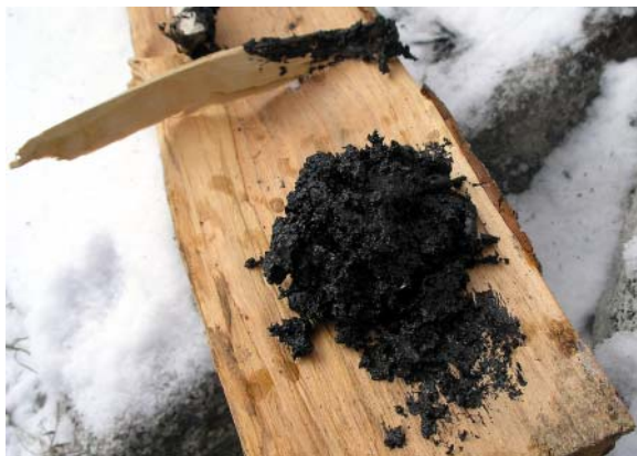
Figure 2.1 Birch tar produced in a one-pot process. Source: Jorre, https://en.wikipedia.org/wiki/File:Birkenpech.JPG . Licensed Under CC BY-SA 3.0.
