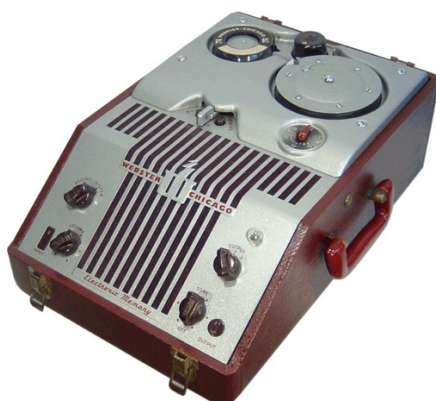
Figure I.2. A wire recorder, the Webster Chicago 180-1 (1949). For a color version of this figure, see www.iste.co.uk/reveillac/recording.zip
