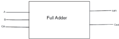
Figure 1.10 Block diagram of a full adder.
