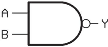
Figure 1.4 Symbol for a NAND gate.
