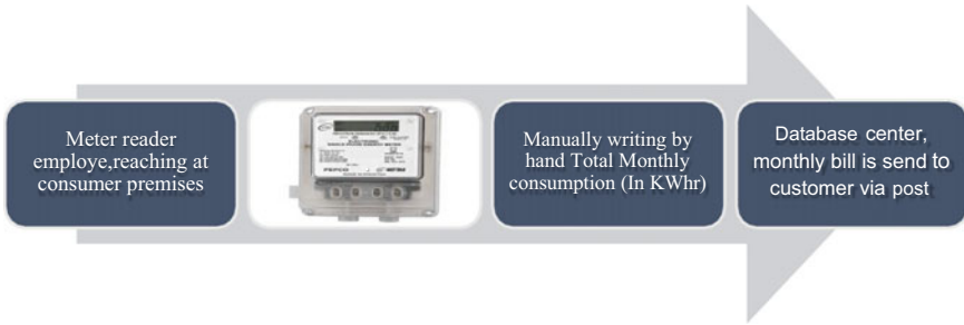
Fig. 2 Current process of data collection, processing, and registering in power distribution companies of Pakistan
