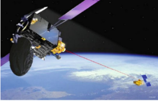
Fig. 1.5 Schematic of intersatellite communications between geostationary Earth orbit (GEO) and low Earth orbit (LEO) satellites for the European Space Agency's (ESA) semiconductor laser inter-satellite link experiment (SILEX) project
