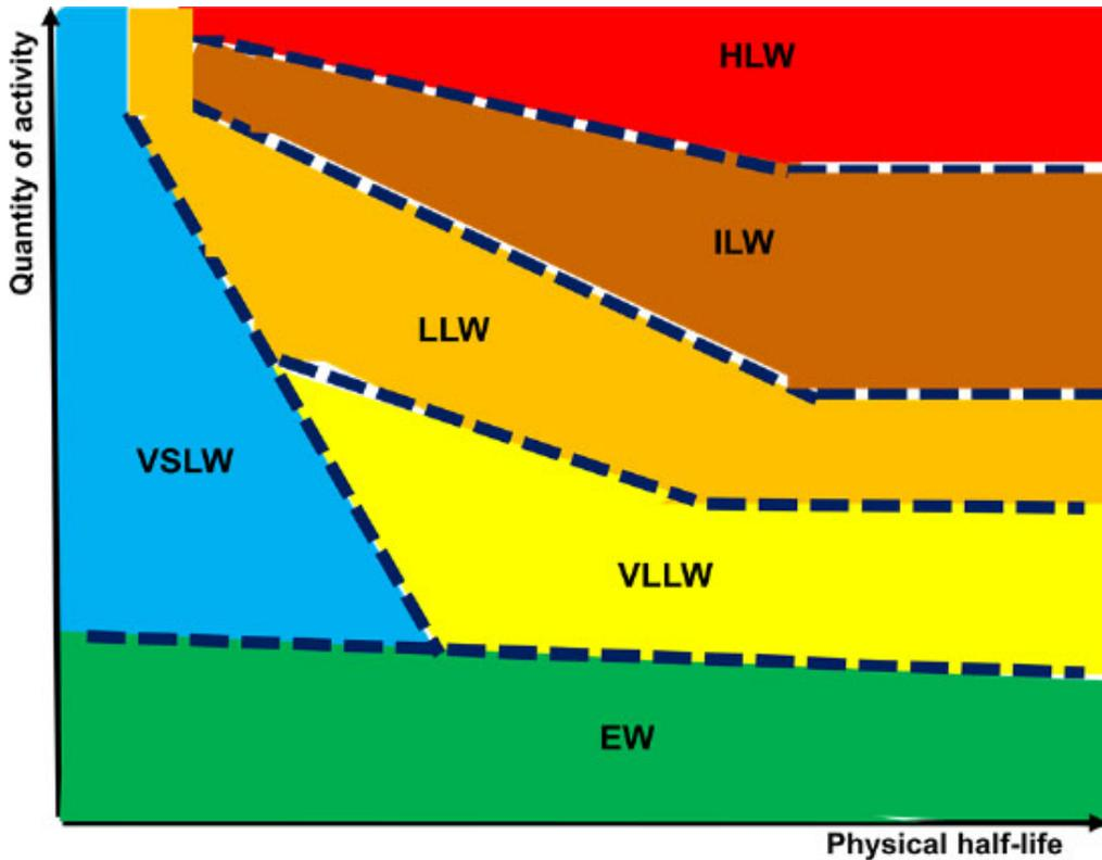
**Figure 1.1.** Proposed IAEA classification of radioactive waste (source: [IAE 09a]). EW: exempt waste; HLW: high-level waste; ILW: intermediate-level waste; LLW: low-level waste; VLLW: very low-level waste; VSLW: very short-lived waste. For a color version of this figure, see [www.iste.co.uk/amiard/radioactive.zip](http://www.iste.co.uk/amiard/radioactive.zip)
