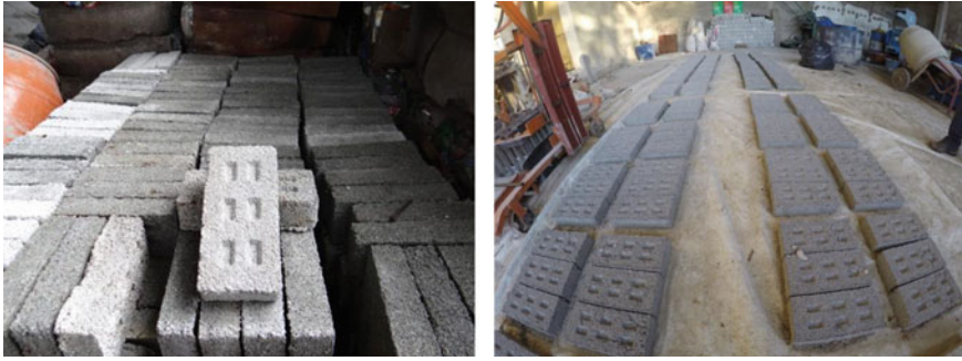
Fig. 10 PET bricks were made from recycled plastic PET bottles in Cordoba, Argentina (Bricks Made from Recycled PET Bottles 2018)
