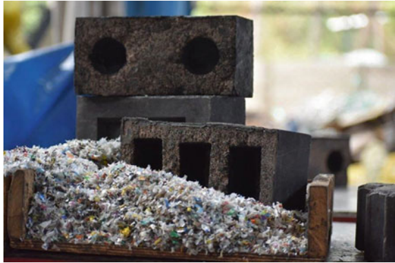
Fig. 8 Silica plastic blocks produced by Rhino Machines (Jo and Park 2006)
