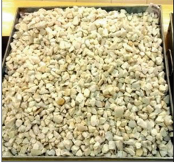
Fig. 2 Recycled PET use as replacement of aggregate (Islam et al. 2016)
