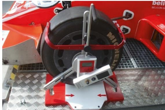
**Table 1.5** Determination of the camber values on the front and rear axle
