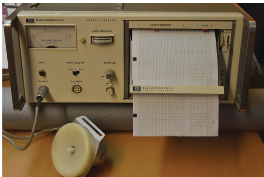
Fig. 1.1 Early model (8020A) of a transportable cardiocograph developed by Hammacher in cooperation with Hewlett Packard, suitable for clinical use. (© Erich Saling)
