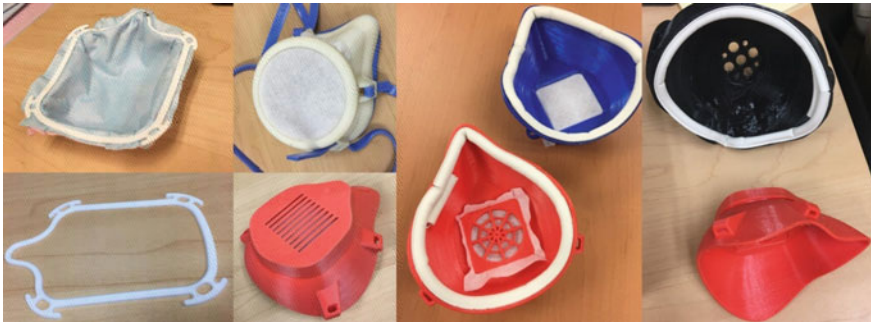
Fig. 1 Various mask designs evaluated or refined at our laboratories, ranging from minimal 3D printed frame-based ones to fully 3D printed filter carriers
