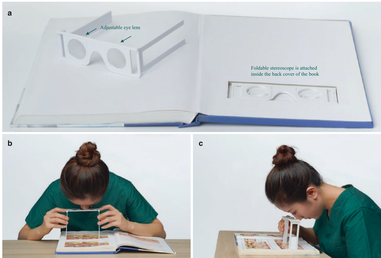
a. Foldable stereoscope is attached inside the back cover of the book. b, c. front view and side view of positioning of the stereoscope.
