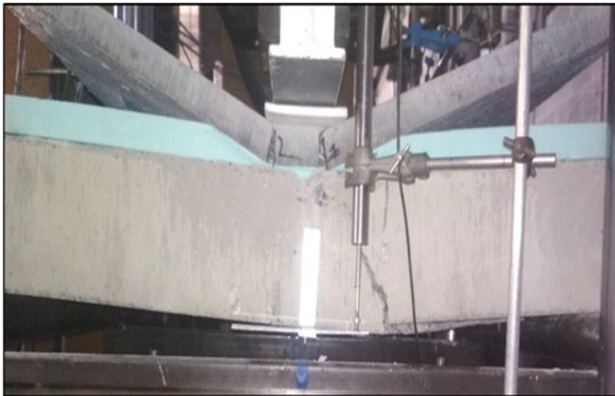
Fig. 18 Failure point of XPS insulated PCSP with top wythe disengaged (Shukla 2019)
