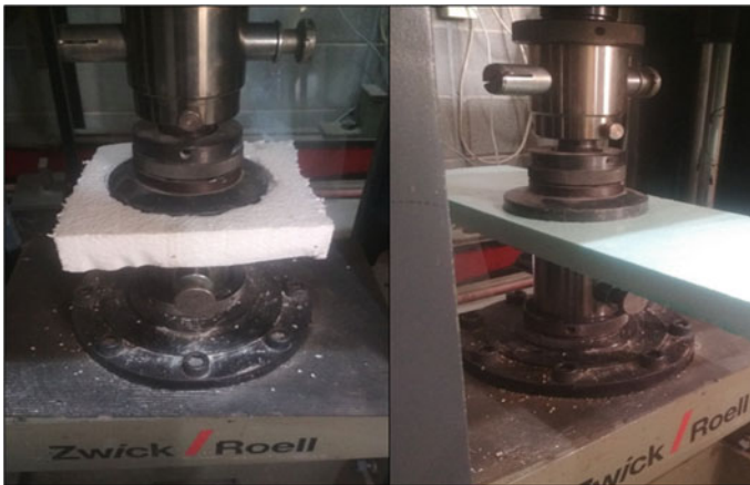
Fig. 4 Compression test on EPS (left) and XPS (right) insulation sheets (Shukla 2019)
