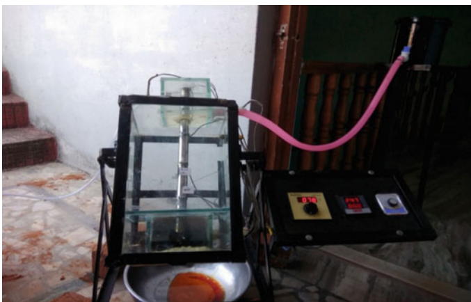
Fig. 2 Experimental setup of heat pipe insulated with glass vacuum chamber
