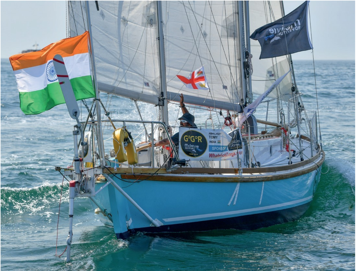
Servo-pendulum system on SV Thuriya at the start of the Golden Globe Race
