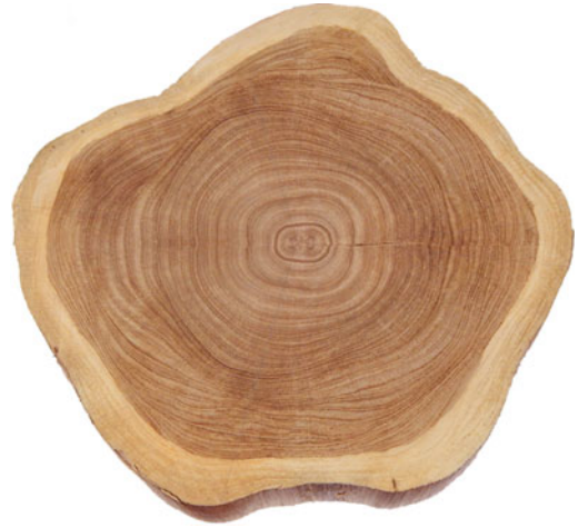
Fig. 1.1 The cross-sectional surface of teak with decorative streaks (growth rings). Photo © P. K. Thulasidas
